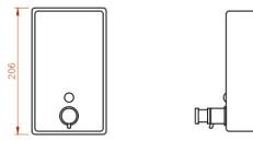
Height: 206mm Width: 121mm Depth: 122mm Weight: 0.6Kg Capacity: 1200ml
